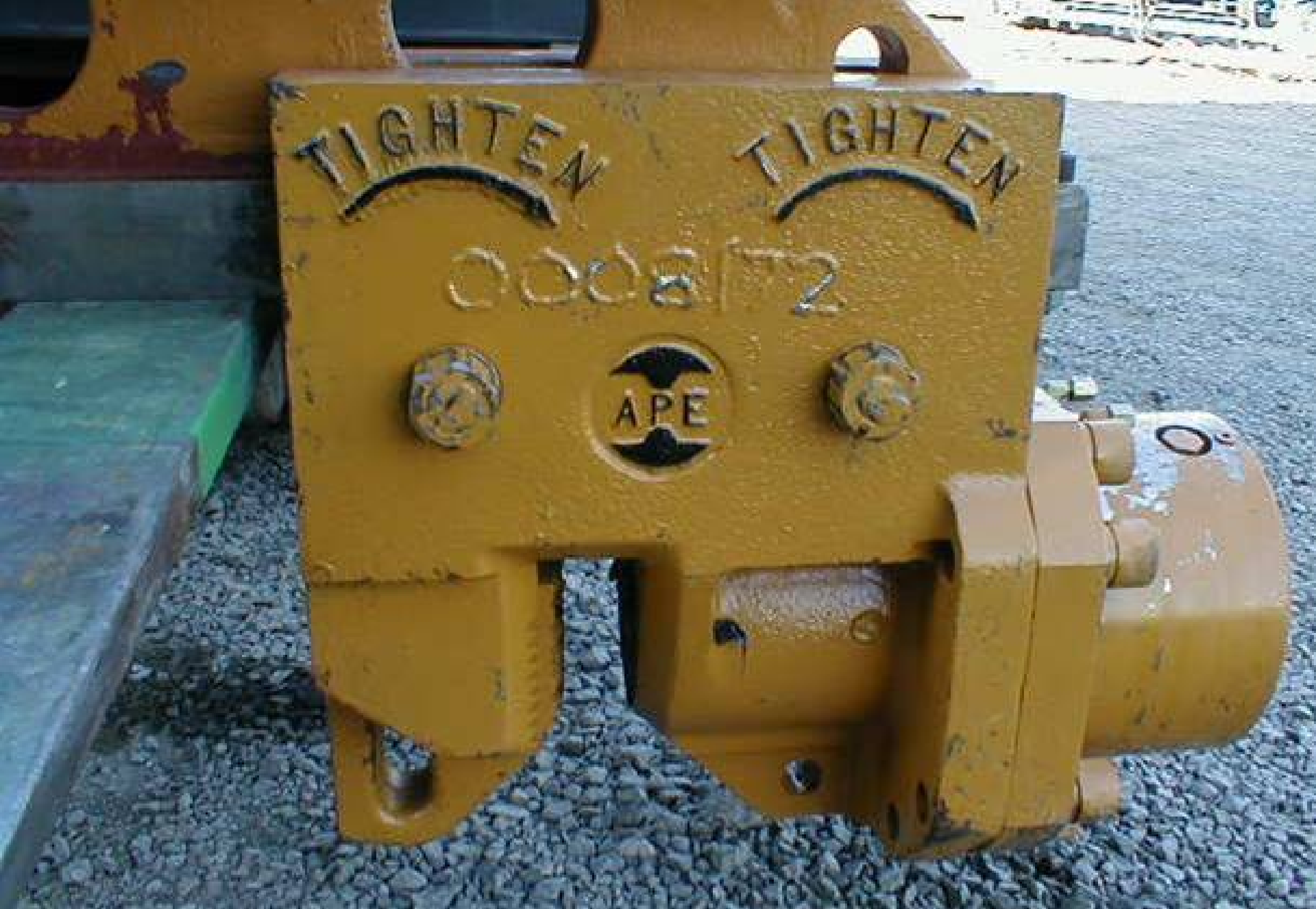
Duel guiding, full six inch slide, check valve clamp, easy to read
